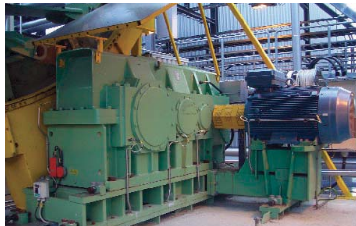
One of two drives for the plant's massive Lime Kiln.
